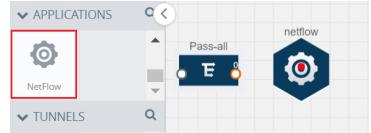
2. Click the NetFlow application and select **Details**. A quick view is displayed for configuring the NetFlow application.
