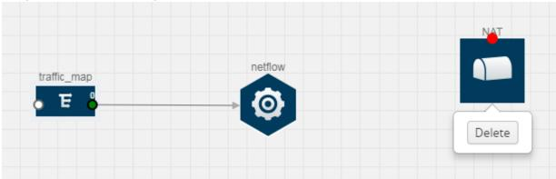
9. Create a link from the v5 NetFlow application to NAT. The link must be configured with the destination IP address of the NetFlow collector and the GigaVUE Cloud Suite V Series node interface. For steps to configure the link, refer to Add Applications to Monitoring Session.
